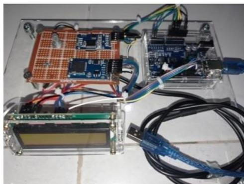
Gambar 5. Hasil rancangan hardware pengukur suhu kalorimeter.
